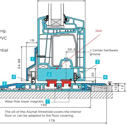
With integrated exterior doors in old construction, the existing stop threshold must be removed. The barrier-free ALUMAT magnet double seal must be fitted into the decorative frame rebate and **sealed on the side.** Either shorten or lengthen the doors with approx. 4 mm gap to the ALUMAT floor profile.
