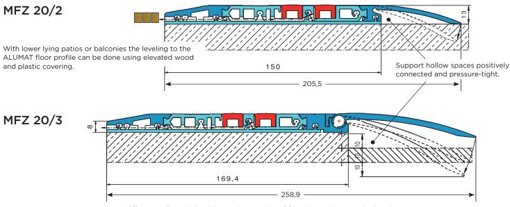
Level differences from higher lying patio covering of from 10 to 30 mm to the interior floor covering can be bridged with the adaptable inclined ramp.
